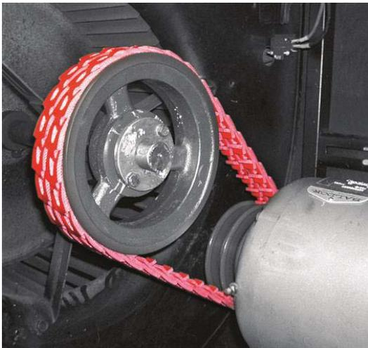
1. One of the best solutions is to use a low-particulate belt. Low-particulate belts are specially engineered so as not to break-down as easy as conventional belts – and they will run smoother and cooler. Most of these low-particulate belts come in the same size and dimensions that the typical drive belts do – so it can be easy to swap them out.
